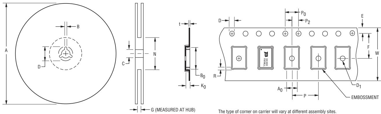
The type of corner on carrier will vary at different assembly sites.
