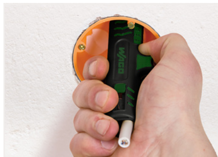
Stripping a cable sheath.
